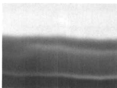
Fig. 3. Surface morphology and edge view of amorphous DLC film viewed under SEM at angle 15^{\circ} degree from normal to surface.
